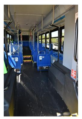
The new low-floor Gilligs, which allow seating for up to 31 passengers and up to two (2) wheelchairs, will be used on the local fixed routes. Easy and efficient mobility device access is provided by a ramp which deploys from the front door.
