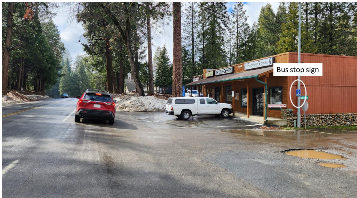
Figure 13 - Example of Bus Stop Sign that is Not Adjacent to the Street and Is Difficult to See
